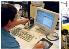
$\begin{array}{c} \textbf{Diameter with the help of laser measurement} \\ \textbf{Dimensions in micrometres ($\mu m$) of milling and drilling before and after} \\ \textbf{machining} \end{array}$
