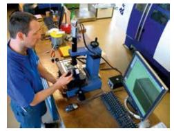
**Digital Optical Systems**Digital measurement and profile comparisons directly from the CAD file
